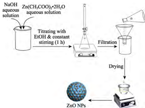
图 1 溶胶-凝胶法制备 ZnO 纳米粒子的过程示意图 [24] Fig. 1 Preparation of ZnO nanoparticles by sol-gel method [24]
