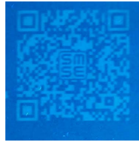
图 6 打印的二维码在 365 nm 紫外灯下照射的效果照片 Fig. 6 Photo of the effect of the printed two-dimensional code irradiated under 365 nm UV lamp
